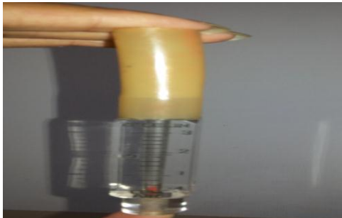
Plate 3: Flow meter for measuring air flow rate
